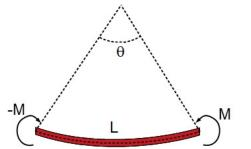
If you bend this multi-colored beam into an arc (right) as shown above, you're looking at the red face (in the y-z plane).
