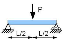
With the axes we've described at the top of the page, this load P is like a weight in y direction. The moment the beam feels is in x because the load P acts at a distance in z away from the pin & roller at the ends. Force in y, distance in z = moment in x
